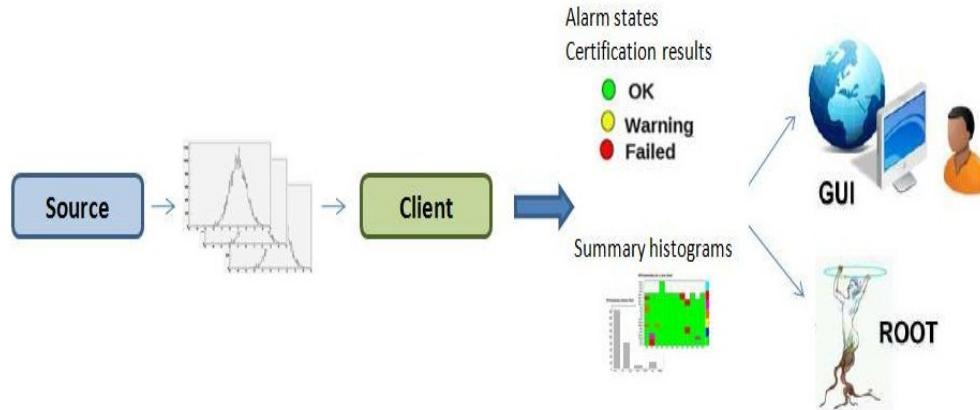
Figure 4.6: Illustration of the source/client structure of the RPC DQM.
