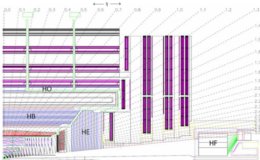
Figure 2.10: Schematic view of the CMS HCAL.
