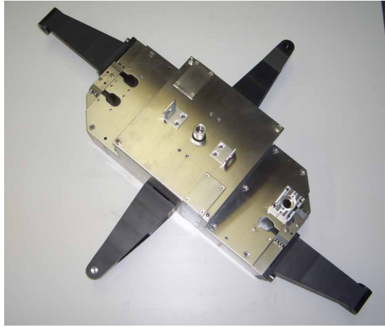
Figure 56: A picture of the new marionette designed for Virgo+ monolithic suspensions. The black dielectric arms are in Peek CF30.
