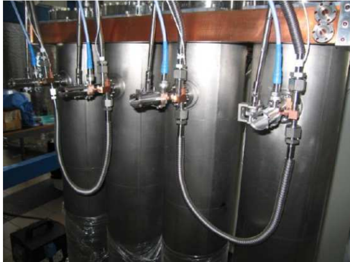
Figure 8.22: Photo of the N-cooling scheme of full Nb 80 MHz QWRs of ALPI.
