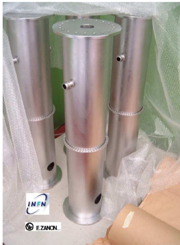
Figure 8.18: The low-beta cavities, in their construction phase
