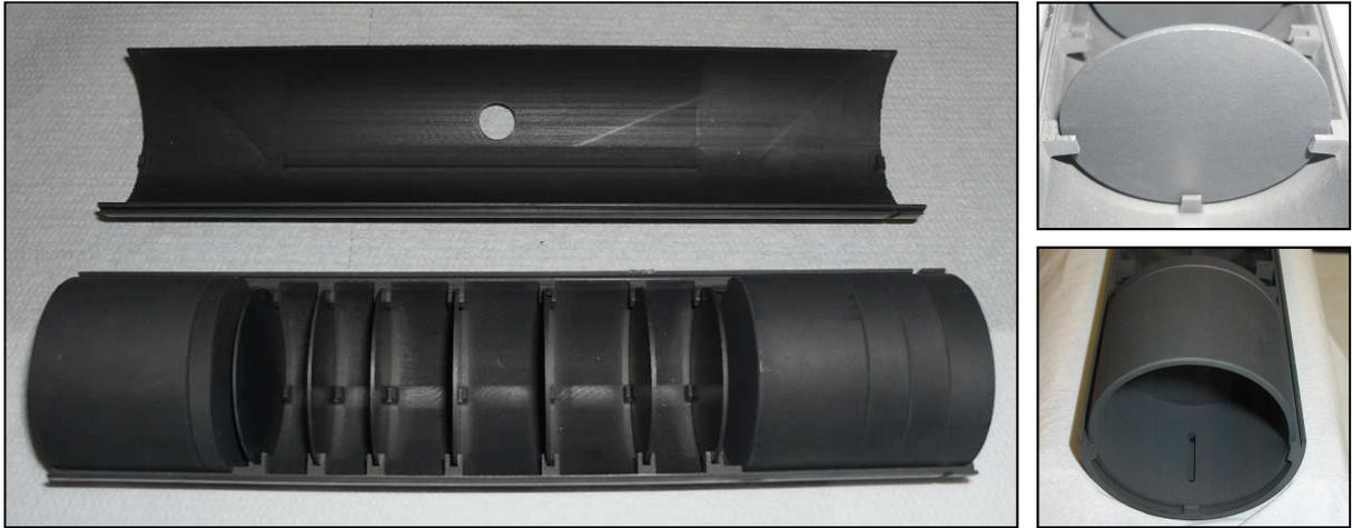
**Figure 5.8:** The full scale SiC SPES target prototype.
