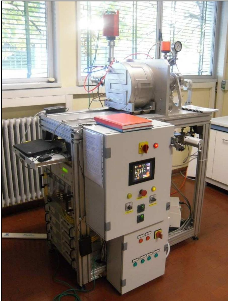
**Figure 5.20:** The LNL furnace for the production of carbides of diameter 40 mm.
