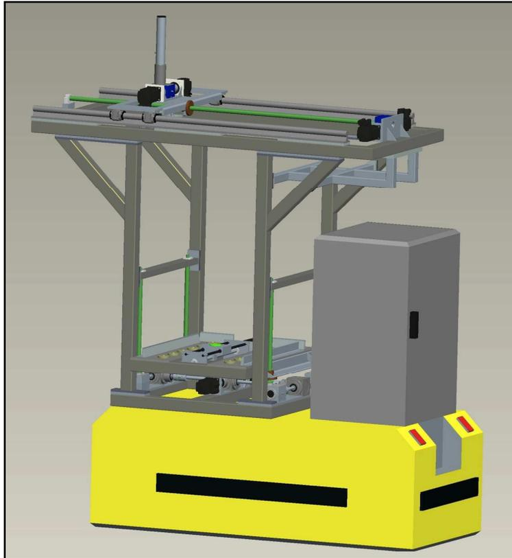
*Fig. 5.20.- The 3D representation of the SPES horizontal handling device. The machine is able to move the target chamber from the lead box to the FE and vice versa. This part of the device will be place over the AGV.*
