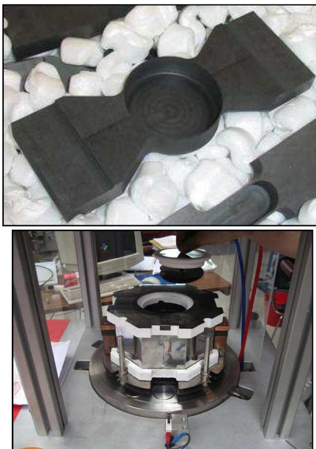
*Figure 5.19: Graphite crucible (left) and screening system (right).*
