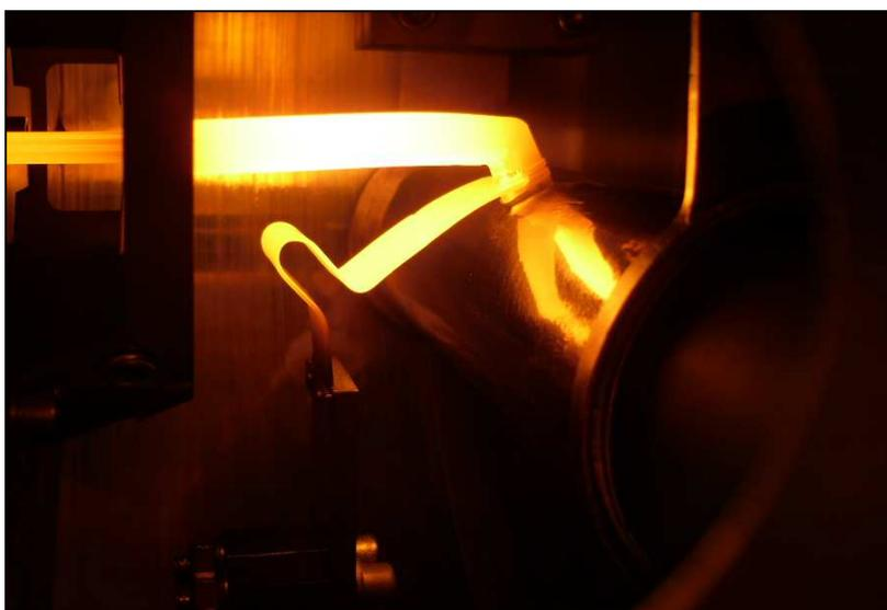
**Figure 5.11:** Picture of the “production target – hot-cavity ion source” assembly heated by an ion source current equal to 200A.
