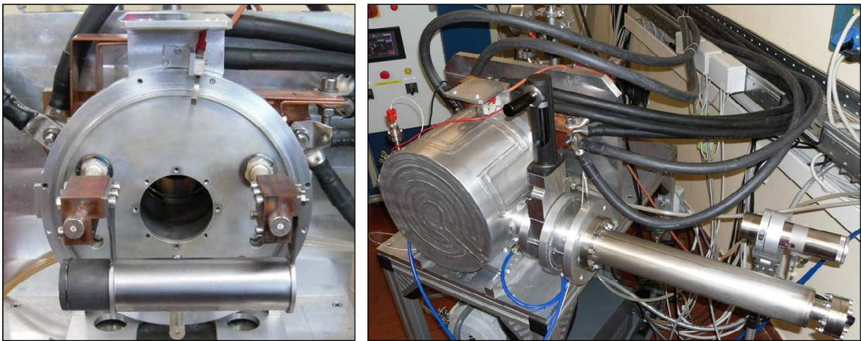
**Figure 5.9:** Target and heating system installed in the vacuum chamber (left); the water-cooled vacuum chamber closed and ready for the high temperature test (right).
