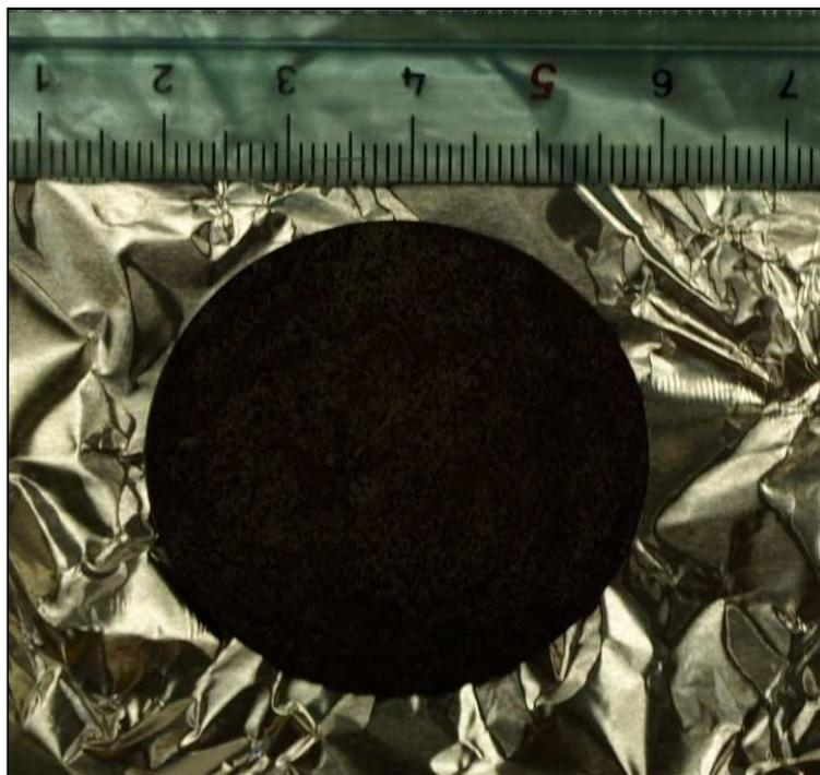
**Figure 5.22:** The 40 mm UC<sub>x</sub> pellet (1 mm thick) after thermal treatment (the average bulk density is about 3 g/cm<sup>3</sup>).
