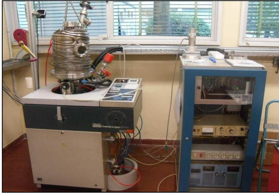
*Figure 5.25: The LNL furnace for pellet thermal characterization.*
