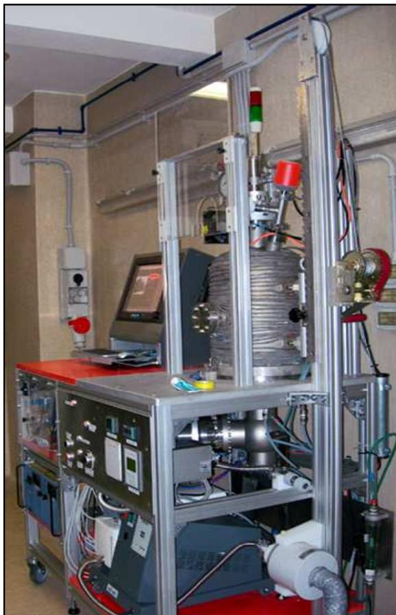
*Figure 5.16: The high temperature furnace for UC<sub>x</sub> production assembled at LNL.*
