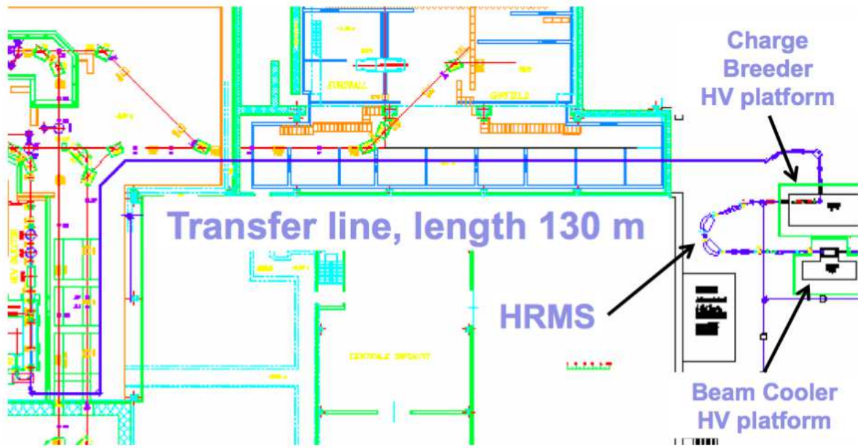
Figure 7.4: Layout of the beam transport line from the Beam cooler to the injection in PIAVE RFQ. The positions of Beam Cooler, HRMS, Charge Breeder and beam transfer line are shown (2010).
